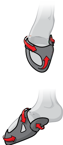
PRESSURE DISTRIBUTION OF 3-FORCE SYSTEM
